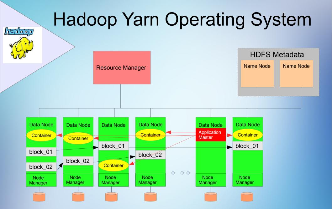
Resource Manager spawns an Application Master for each job which in turn negotiates for resources with Node Managers and monitors execution. Containers are individual execution threads managed by the Application Master.
